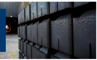
For many years our Bell Bay aluminium operation has been pioneering a coating for carbon anodes to help reduce consumption, and therefore waste. Through the Pioneer Portal, the team sought a world-first solution to automatically apply their protective coating on baked carbon anodes.
